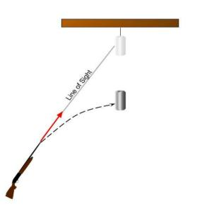
A small can is hanging from the ceiling. A rifle is aimed directly at the can, as the figure illustrates. At the instant the gun is fired, the can is released. Ignoring air resistance: show that the bullet will always strike the can. regardless of the initial speed of the bullet. Assume that the bullet will strike the can before it hits the ground.
